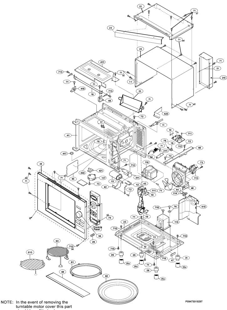
turntable motor cover this part should be refitted using screw connection: 5028 14 53-00/6 (710)
